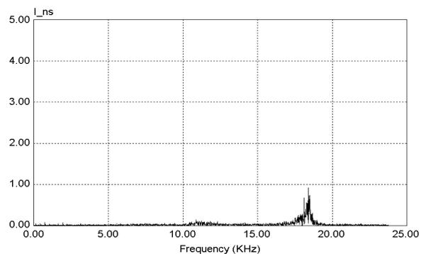
Figure 8. The spectrum of neutral current after compensation
