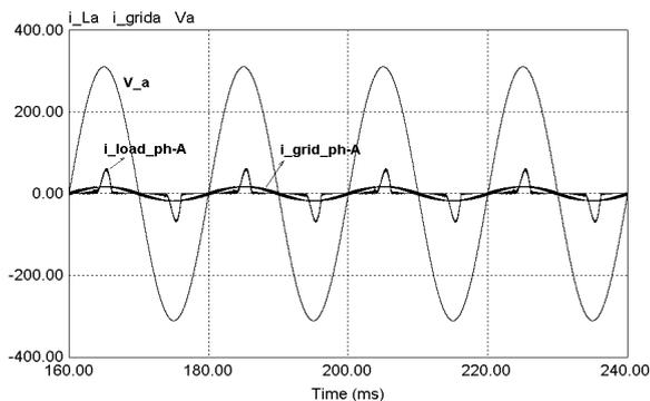
Figure 6. Grid voltage, load current and grid current
